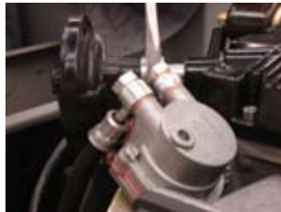
The picture above shows the fuel return line connection location.
